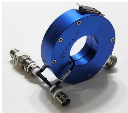
Figure 11: CT Around Measurement Loop ( 81\ \text{nH} ) and 50\ \Omega Resistor
