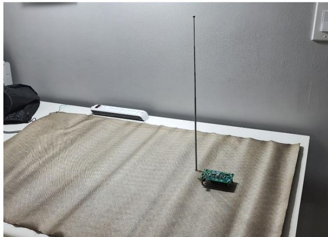
Figure 25: Comb generator (3 MHz) with 18" antenna on ground plane
